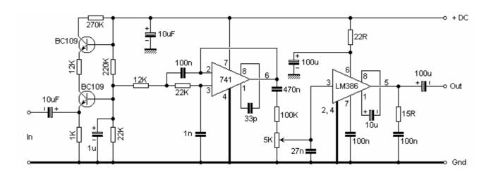
Audio taken from your receiver is fed to the pre-amp which consists of the two BC109 transistors and
